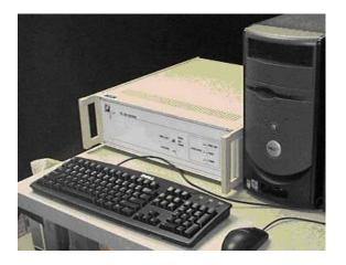
The **ITS23S** is an updated version the ITS10S coherent receiver system originally developed in 1994 by NorthWest Research Associates. This model is physically and electronically similar to the <u>ITS33S Three-Band receiver</u>, lacking only the L-Band (1067 MHz) capability.
