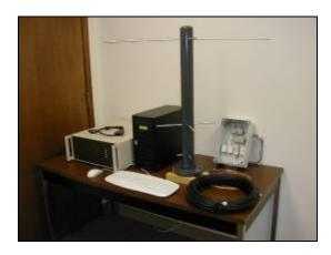
The **ITS30S** is a three-frequency version of the ITS10S receiver originally developed in 1994 by NorthWest Research Associates. This model was developed in anticipation of the three-frequency CERTO class beacons. The ITS30S Coherent Receiver System is used for ionospheric research and is designed to measure ionospheric effects on signal phase and intensity from satellite beacons operating at 150, 400 and 1066.67 MHz (nominal).
