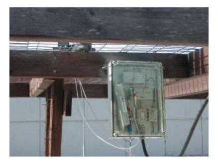
In the configuration shown above, in Bellevue WA, the VHF preselector being tested was narrow enough to prevent saturation of the LNA, but the insertion loss of that filter was 7 dB. This meant that the receiver noise figure at VHF was nearly 10 dB.
